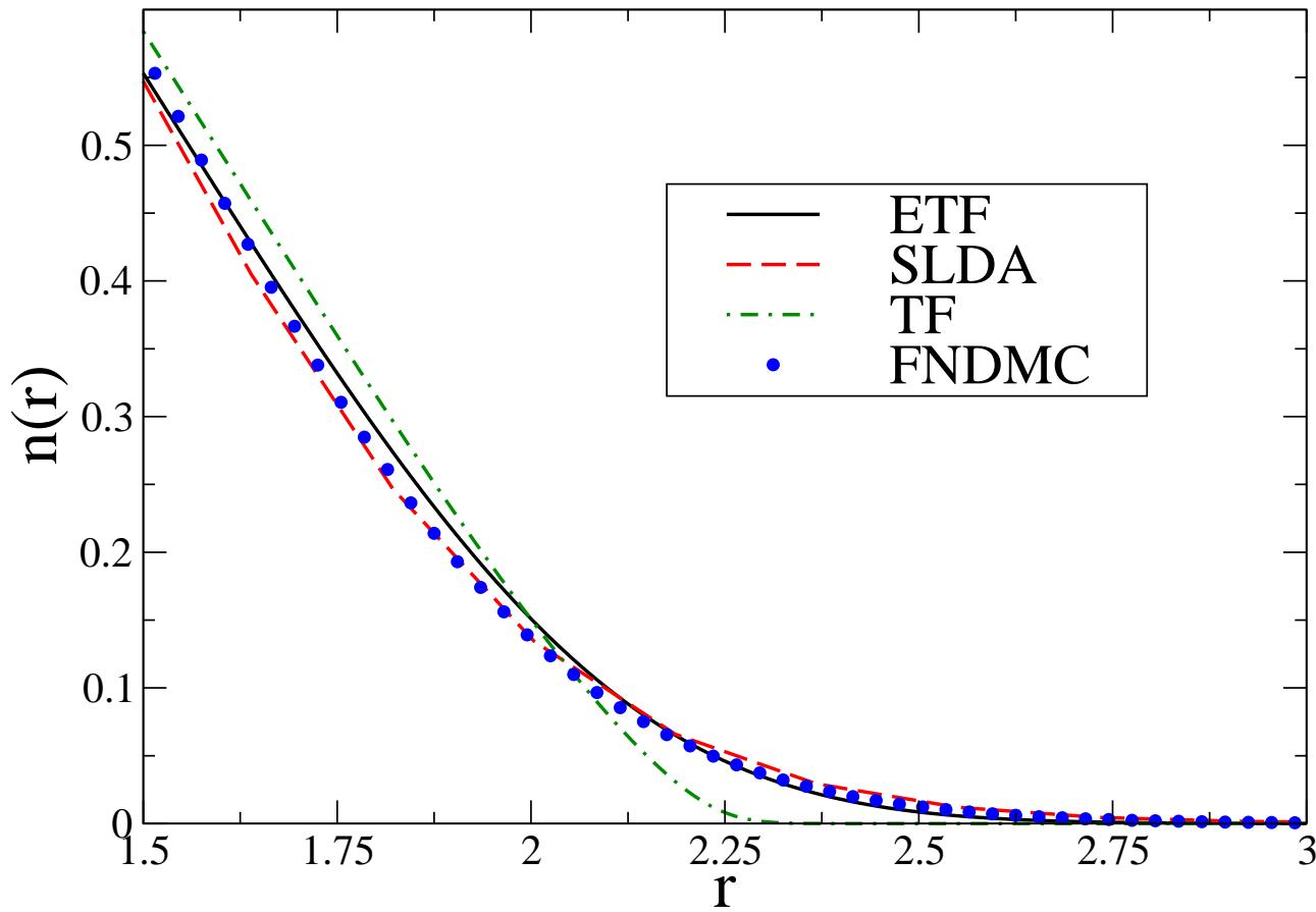
Zoom of the density profile  $n(r)$  for  $N = 20$  fermions near the surface obtained with our ETF (solid lines), Bulgac's SLDA (circles) and FNDMC (circles). Lengths in units of  $a_H = \sqrt{\hbar/(m\omega)}$ . [L.S., F. Ancilotto and F. Toigo, Laser Phys. Lett. 7, 78 (2010).]
