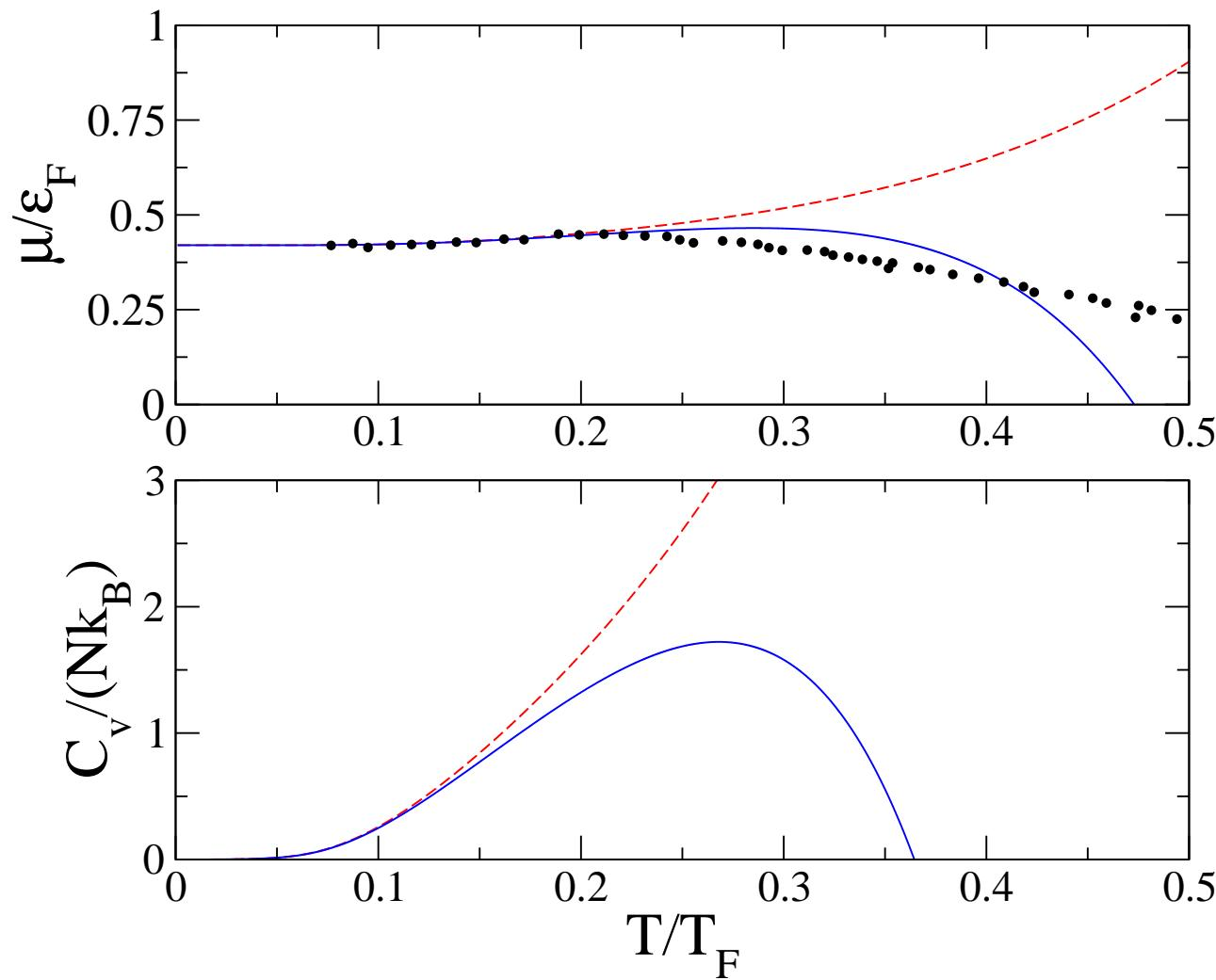
Chemical potential  $E$  and heat capacity  $C_v$  of the unitary Fermi gas as a function of the temperature  $T$ . **Dashed line:** ST with  $\lambda = 0$ . **Solid line:** ST with  $\lambda = 0.27$ . Circles: Monte Carlo results of A. Bulgac, J.E. Drut, and P. Magierski, PRL **99**, 120401 (2007). [L.S. and F. Toigo, very preliminary results.]
