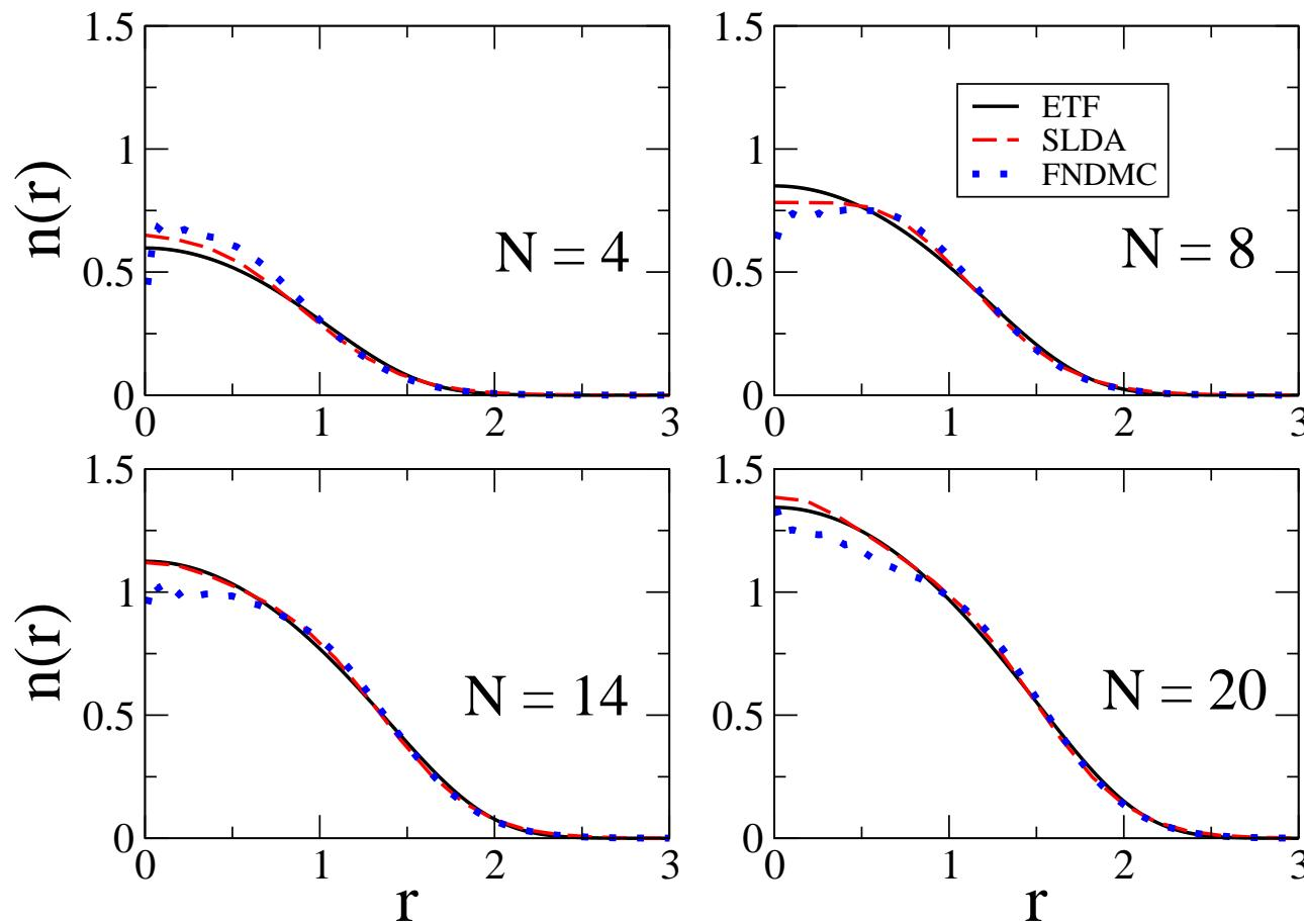
Unitary Fermi gas under harmonic confinement of frequency  $\omega$ . Density profiles  $n(r)$  for  $N$  (even) fermions obtained with our ETF (solid lines), Bulgac's SLDA (dashed lines) and FNDMC (circles). Lengths in units of  $a_H = \sqrt{\hbar/(m\omega)}$ . [L.S., F. Ancilotto and F. Toigo, Laser Phys. Lett. **7**, 78 (2010).]
