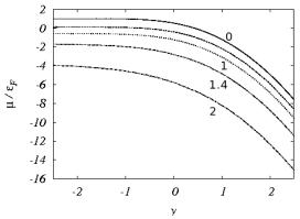
Scaled chemical potential  $\mu/\epsilon_F$  as a function of the adimensional interaction strength  $y=1/(k_Fa_s)$  for different values of the scaled Rashba velocity:  $v_R/v_F=0$  (solid line),  $v_R/v_F=0.7$  (long-dashed line),  $v_R/v_F=1$  (short-dashed line),  $v_R/v_F=1.4$  (dotted line),  $v_R/v_F=2$  (dashed-dotted line). Here  $\epsilon_F=v_F^2/2$  is the Fermi energy and  $v_F=(3\pi^2n)^{1/3}$  is the Fermi velocity.
