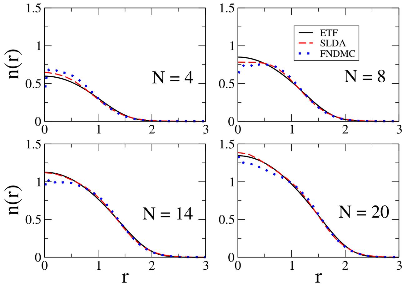
Unitary Fermi gas under harmonic confinement of frequency  $\omega$ . Density profiles  $n(r)$  for  $N$  (even) fermions obtained with our ETF (solid lines), Bulgac's SLDA (dashed lines) and FNDMC (circles). Lengths in units of  $a_H = \sqrt{\hbar/(m\omega)}$ . [L.S., F. Ancilotto and F. Toigo, LPL **7**, 78 (2010).]
