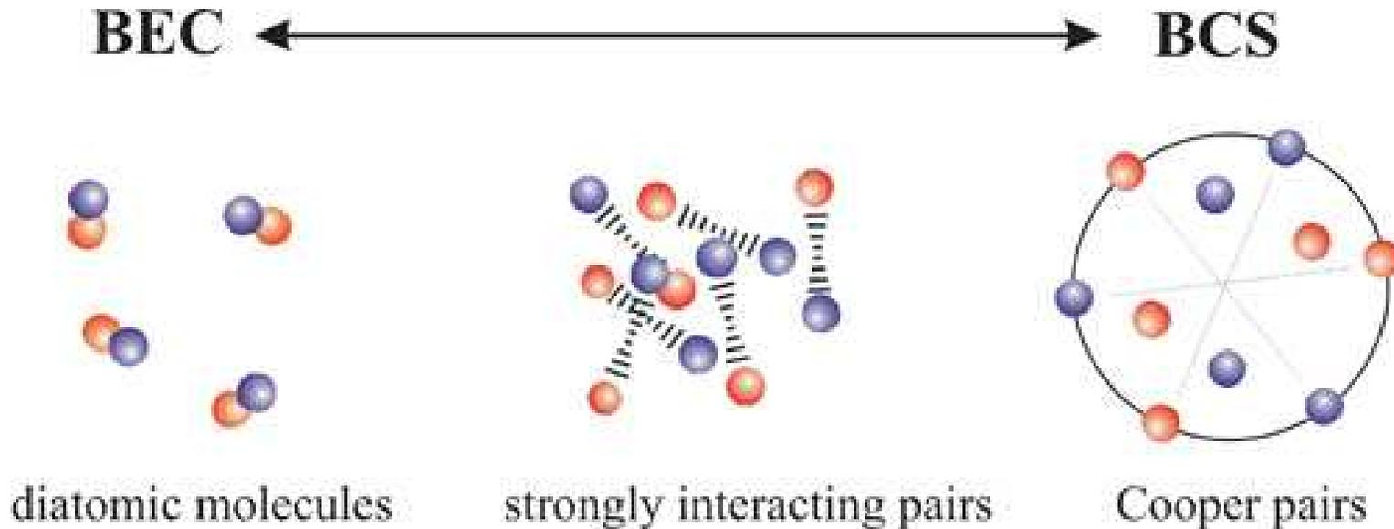
This crossover is obtained by changing (with a Feshbach resonance) the s-wave scattering length  $a_F$  of the inter-atomic potential:
