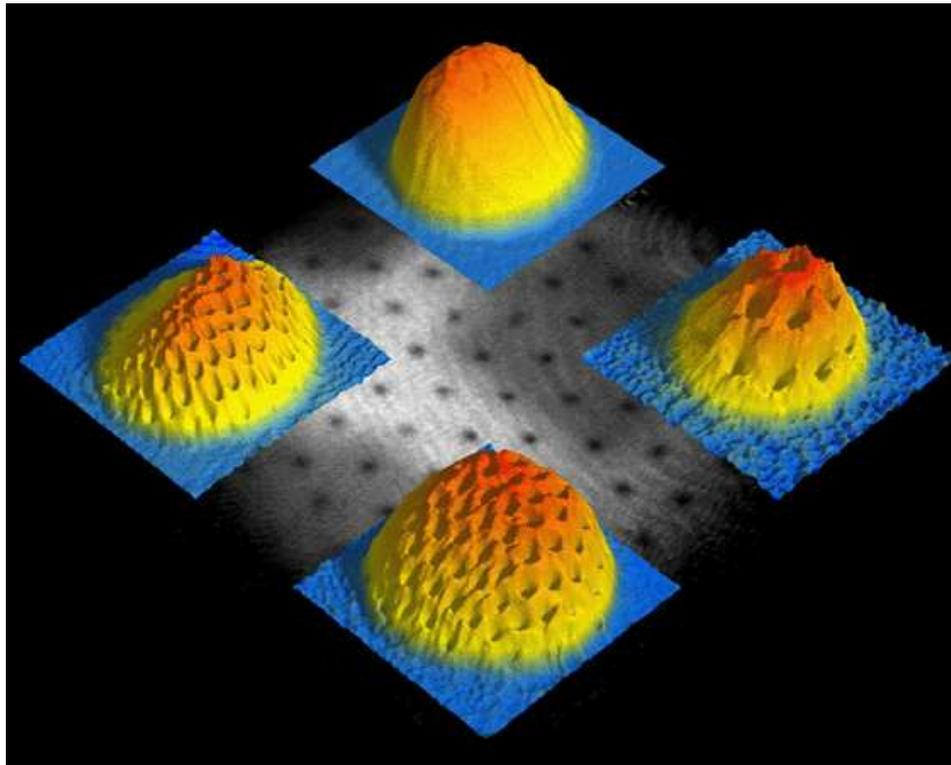
Formation of quantized vortices in Bose-condensed gas of  $^{87}\text{Rb}$  atoms. The number of vortices increases by increasing the rotational frequency of the system.
